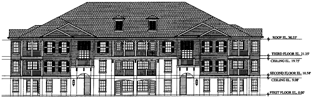
① BUILDING TYPE ONE - FRONT/REAR ELEVATION
