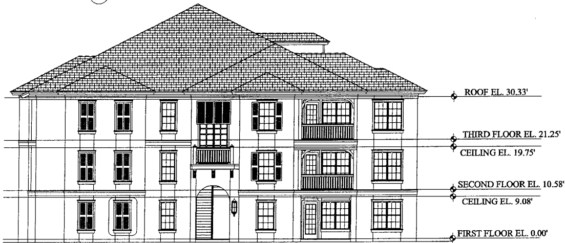
② BUILDING TYPE TWO - LEFT ELEVATION
